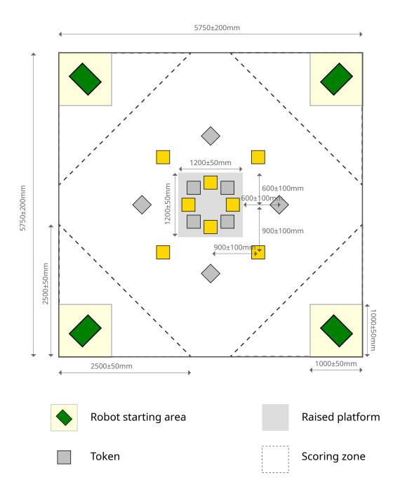
Figure 2: A bird's-eye view of the arena. All dimensions are in millimetres.
