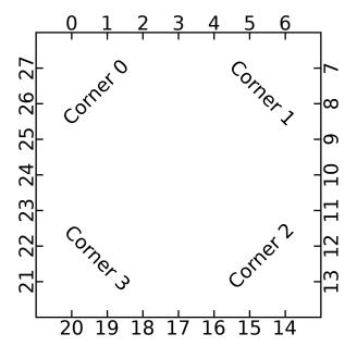
Figure 4: Twenty eight arena wall markers are positioned around the perimeter of the arena with the marker codes incrementing in a clockwise fashion. The corners are counted in a clockwise fashion, with corner 0 being the corner closest to arena marker 0.
